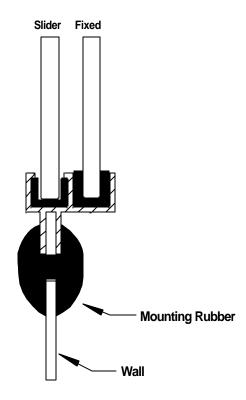
The Series 900 is a commercial quality two channel designed window that is installed with a lock rubber gasket. This window consistently meets the demands of the toughest operating conditions. The Series 900 is most specified for use in heavy equipment, commercial cabs, and marine windshields.
