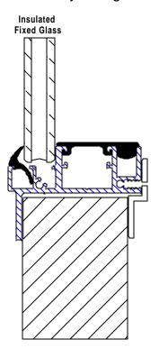
Series 1800 Motion Windows is designed for 1/2" dual pane glass-providing many product benefits including superior insulation, minimal air and wind intrusion, reduced condensation, and noise reduction. They are manufactured with solid tempered glass, true double seals, anodized perforated aluminum spacers, and high quality two-part absorption media for a long, trouble free life.
