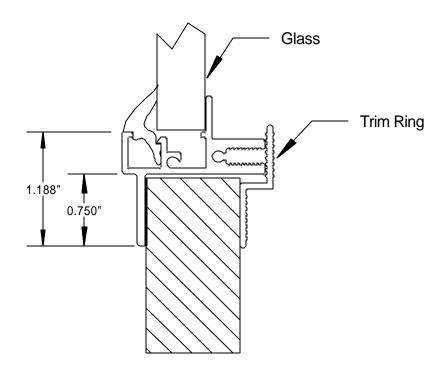
The Series 1250 is a stationary (fixed) clamp ring window designed specifically for marine applications.
