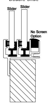
The Series 1200 is a clamp ring window designed specifically for marine applications. It offers customers the choice of forward (front to rear), rear (rear to front) or double -sliding glass configurations. A unique high-back slider track design and ample face slots give the Series 1200 quick water evacuation and excellent slide capability in the most severe conditions.
